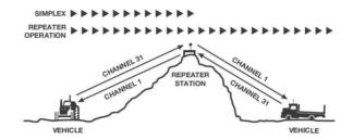
Your XRS Connect radio allows you to enable or disable Duplex mode on individual repeater channels. In this way any repeater channels that are not being used with repeaters in your area can be used in Simplex mode for normal direct radio-to-radio communications.
