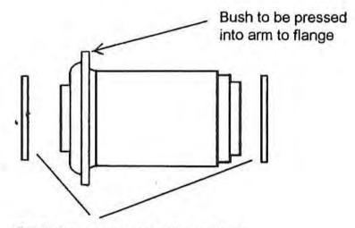
NOTE: Grease to be applied to bush side of washer and face of bush.
