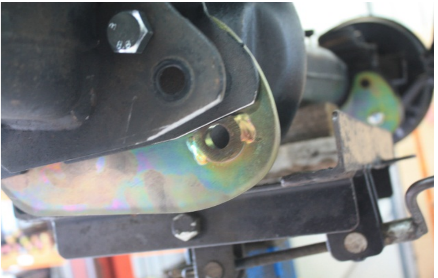
Figure 2: NOTE Half washer hard against cut diff plate
