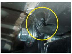
7. Using an assistant, lift side step into position over U-Bolts and attach nuts, flat and spring washers supplied.
