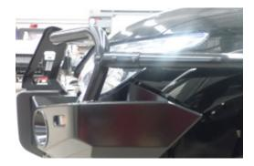
12. Ensure all mounting hardware for checkerplate is tight.
