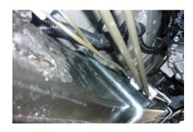
4. Position front U-Bolt over front captive nut as shown in pic
