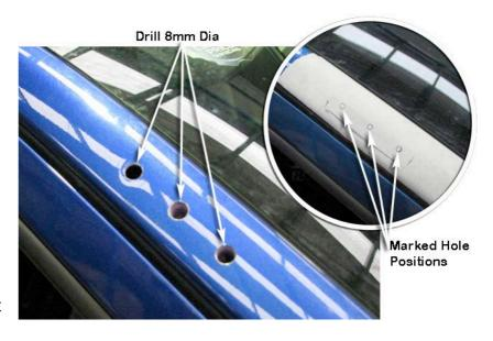
Install the plastic inserts (Item 6) into the upper mounting bracket holes in the A-pillar.
