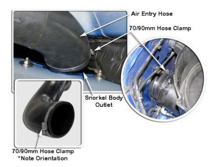
Install the black hose clamp (Item 12) loosely over the base of the air ram assembly (Item 2).
