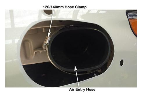
Apply lubricant to the inlet of the air entry hose (item 11).
