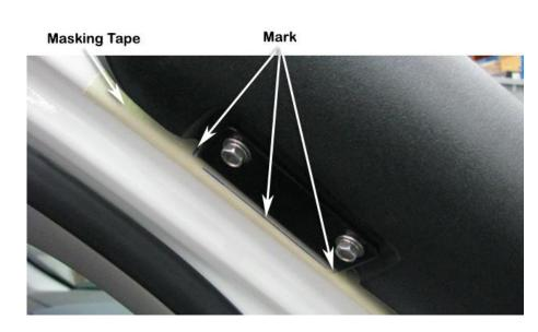
Position the upper mounting bracket onto the A-Pillar and align the bracket with the marked bracket outline. Mark the three mounting hole positions with a felt tip pen.
