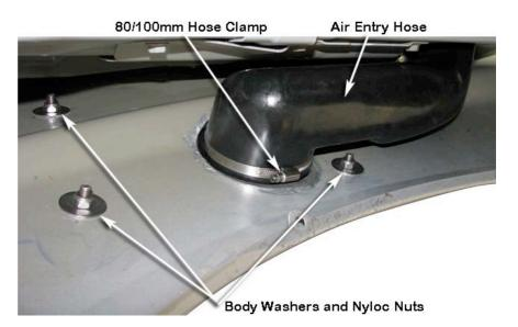
Install the black hose clamp (item 16) loosely over the base of the air ram assembly (item 2). Install the air ram assembly onto the snorkel body.
