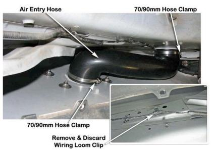
Install the black hose clamp (Item 16) loosely over the base of the air ram assembly (Item 2).
