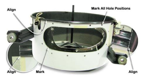
**16** Use a 4.0mm drill bit to drill all twelve marked hole positions.
