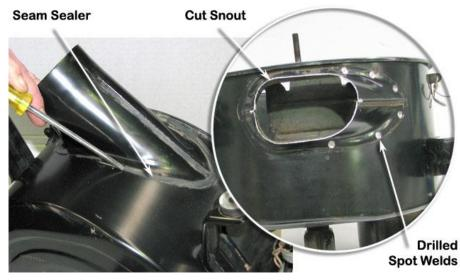
**13** With all the spot welds drilled out use a small pry bar or flat blade screwdriver to remove the inlet snout from the air cleaner housing. Take care to avoid damaging the air cleaner housing.
