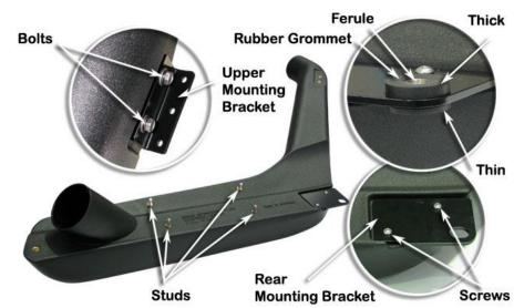
Apply loctite 243 to the two 6mm button head cap screws (item 8) and secure the rear mounting bracket (item 7) to the snorkel body as shown.
