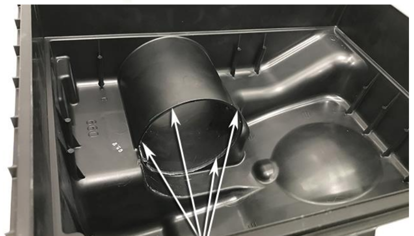
Remove End Section of Pre Spinner Chamber
