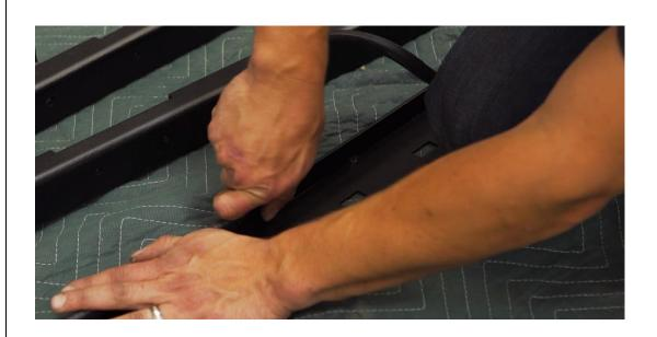
4. Fit Pinch weld to short edge of roof rails. Trim excess off with side cutters
