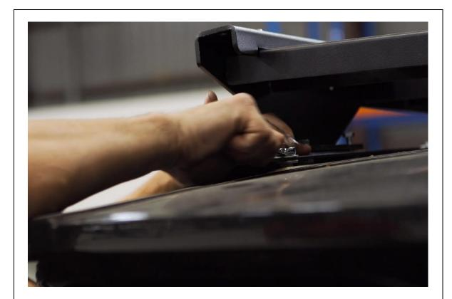
13. Position rack, and ensure all fasterns are threaded, then torque down each M8 and M6 fastener
