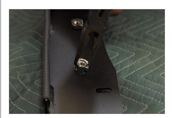
5. Fit nutserts as shown in both rails (6 per rail). You can use needle nose plyers or screwdriver to push one end of cage in from side
