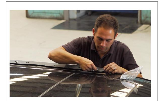
7. Loosely fit Rails to roof with M6 Hex bolts and mud guard washers. Do not torque down yet. 6 per side
