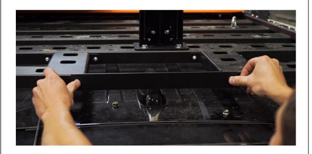
14. Fit rear secure bar with M6 x 25 button head cap screws washers and flange nuts and torque down
