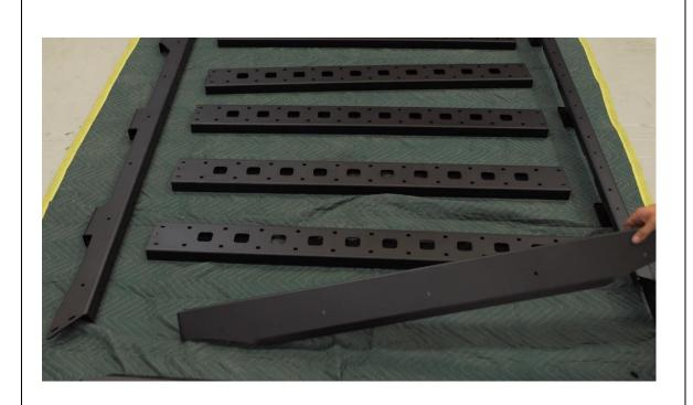
10. Bolt rest of rack together with M6 x 25 button head cap screws, washers and flange nuts
