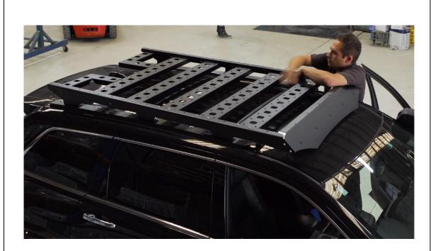
12. Loosely fit M8 bolts and washers through rack into nutserts fitted to steel rail
