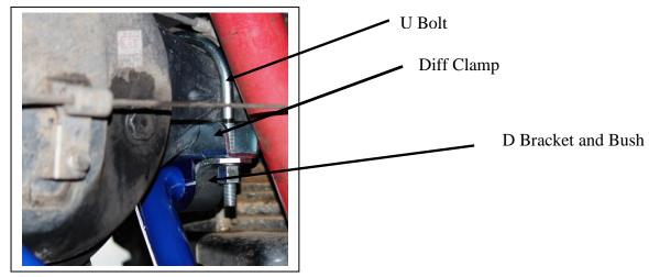
3. If the Diff has Factory brackets fit the bar with the D/Brackets and Bushes supplied.
