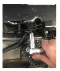
61. Mount the front intrusion bar using the factory bolts.
