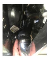
45. Slide the intercooler clamps back into place over the PWR intercooler outlets and fasten the intercooler hose clamps firmly into place.
