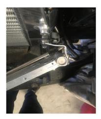
51. Lower the factory air condenser back into place.
