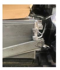
52. Bolt in the air condenser passenger side mount using the PWR supplied M6 medium Allen key bolt and big washer provided.
