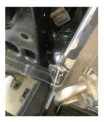
55. Refit the 2 factory bolts to the transcooler lines bracket on the passenger side.
