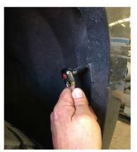
Unscrew screws on top of the radiator support.
