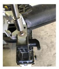
42. Refit bracket to the PWR intercooler using the supplied PWR M6 short Allen key bolt and washer provided.
