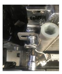
54. Twist the transmission cooler into the bracket locator on the passenger side to lock the transcooler into place.
