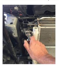
Unscrew screws holding the air condenser and transmission hard lines in place.
