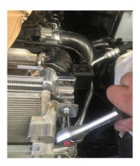
53. The driver's side mount requires the use of the PWR supplied billet spacer, 32mm M6hex head bolt and big washer..
