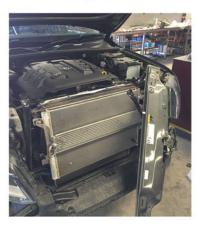
27. Remove the visible screws holding the air condenser, intercooler and transmission cooler in place.
