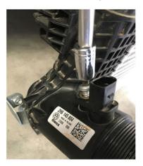
40. Refit sensor on bottom outlet on the new PWR intercooler using the PWR provided M6 short Allen key bolt.
