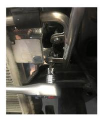
56. Tighten the M6 hex head bolt with a open end spanner on the trans cooler mount.
