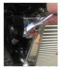
47. Click on the factory sensor plug on the bottom passenger side outlet.
