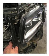
26. Once this is all done retain the bonnet release cable in place and twist the radiator top support cover to the passenger side to give enough access to the cooling products. Be careful not to damage the front of the car, allow for some protection under the radiator support panel.
