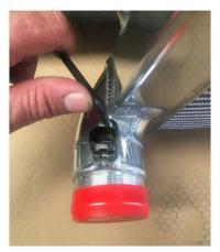
41. Remove bottom factory transmission cooler line bracket from the factory intercooler.
