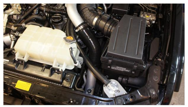
• Fit hose tails and hoses to catch can with clamps supplied.
