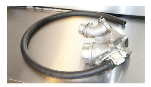
• Fit 900mm long 19mm hose to hose tail on rocker cover outlet with clamp supplied.
