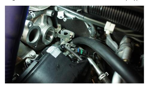
• Bolt turbo air intake, compressor outlet back on to turbo.
