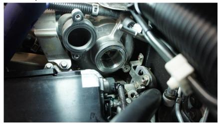
Remove plastic breather on turbo air intake. Remove 'o'ring from plastic breather. Fit 'o'ring to billet aluminium adaptor supplied. Bolt the aluminium adaptor to turbo air intake with factory bolts. Fit hose tail supplied to adaptor. Fit 950mm long 19mm hose to hose tail with clamp supplied.
