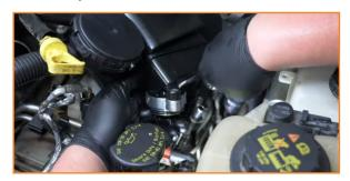
18. Install the adapter and hoses to the back end of the air-oil separator. Make sure the O-ring has not fallen off the bottom of the adapter. The image below was taken with the separator out of the vehicle for a clearer representation.
