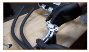
15. Lift the air-oil separator and drain some excess oil. Clean the housing once the oil has been drained.
