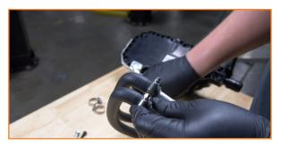
14. Grease the O-ring groove on the aluminum adapter and place the thin O-ring within the groove. This was done outside the vehicle for a clear representation.
