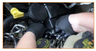
17. Lubricate the new O-ring and install the Mishimoto adapter to the bottom of the air-oil separator.
