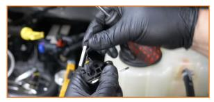
Replace the stock metal bracket attached to the fuel line retaining clip with the provided Mishimoto bracket.
