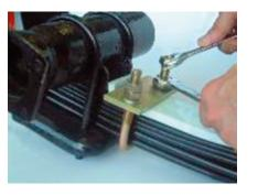
5a. Install the longer U bolt through the "T" shaped end of the Load Plus, including the curved leaves of the spring.
