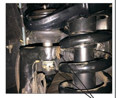
Strike hub knuckle to dis-lodge ball joint. Note - remove and re-fit safety clip.
