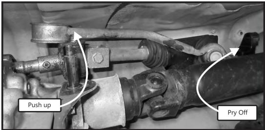
11. Push the gearshift lever arm up over the top shifter mechanism which will allow enough access to pry the rear shifter block off the end of the shaft. (Fig 8).
