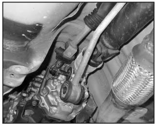
5. Remove the Gear shifter 12 mm nut as shown in (Fig 3).
