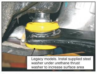
Fig 3 - right-hand control arm, outside view.
