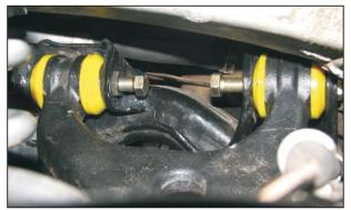
Fig 4 - right control arm, side view.
