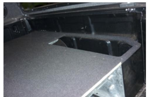
6. Place strengthening brackets in position as shown against side of drawer frame under thin section of top panel.
