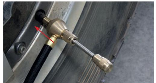
5. Push valve remover back in and screw in a clockwise direction until valve is tight.
