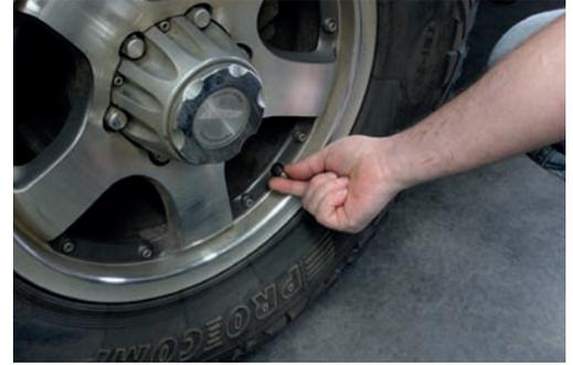
2. Attach Speedy Deflator to valve stem by supporting hose collar and rotating the valve stem adaptor in a clockwise direction.
