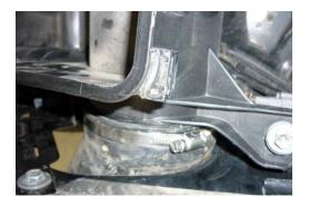
Check all hose connections and air box for potential leaks and seal as required.
