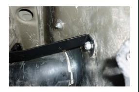
13. Attach rubber joiner to snorkel with outlet towards front of hole in engine bay and secure with hose clamp provided.
