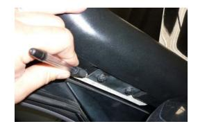
11. Hold bracket in position previously marked on pillar and mark mounting holes.
