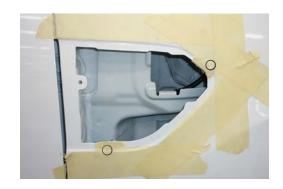
5A. Drill 16mm mounting holes using a step drill. De-burr and rust-proof exposed metal.
