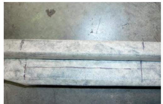
15. Remove section of trim by drilling a series of 3.5mm holes and cutting between holes to create a slot.
