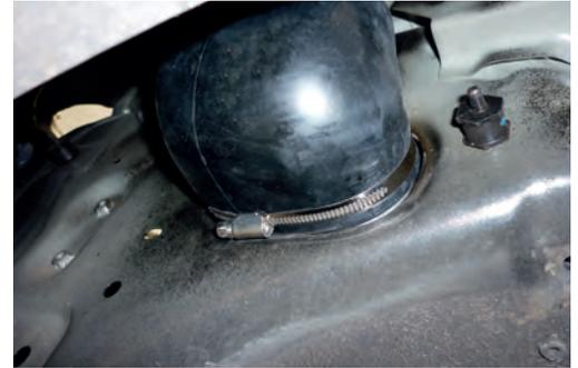
22. Attach snorkel body to mudguard using M8 Nylcok nuts and Bowdy washers, making sure snorkel outlet engages with rubber joiner and secure with hose clamp.
