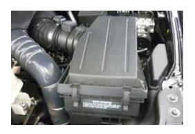
24. Remove intake air duct from air box.
