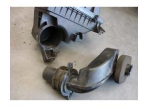
25. Install adaptor to air box. Make sure that cut out is aligned with air intake hole in air box then Pin in place with self tapping screw provided.
