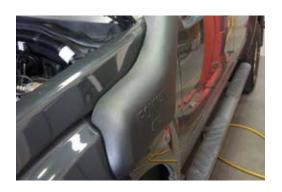
16. Secure inner guard duct to snorkel using self tapping screw provided and recheck connection to make sure duct is sealed properly.
