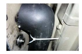
17. Attach snorkel to pillar mounting bracket using M6 Bolts provided.
