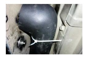
29. Apply a liberal amount of sealant to outside of snorkel outlet and inside of inner guard duct to ensure a water-tight seal.
