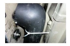
32. Attach snorkel to pillar mounting bracket using M6 Bolts provided.
