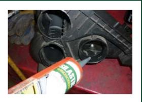
21. Seal hole in air box as shown.
