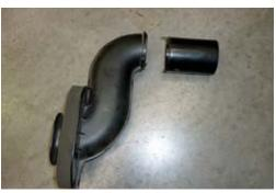
20. Apply a liberal bead of silicone sealant to inside of air entry hole in air box. Fit round section removed from round air entry duct in previous step to air entry hole flush with inside of air box and secure with self tapping screw.
