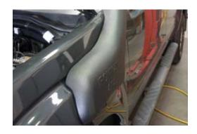
38. Attach snorkel to pillar mounting bracket using M6 Bolts.
