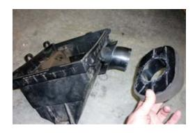
34. Apply a liberal amount of sealant around intake duct inside and outside of air box to create a water tight seal.
