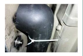
36. Apply a liberal amount of sealant to outside of snorkel outlet and inside of inner guard duct to ensure a water tight seal.
