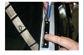
10. Apply silicone sealant to holes, insert mounting plugs and attach mounting bracket to pillar using self tapping screws provided.
