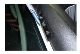
9. Hold mounting bracket against pillar in position previously marked and mark three mounting holes and drill to 7.5mm.
