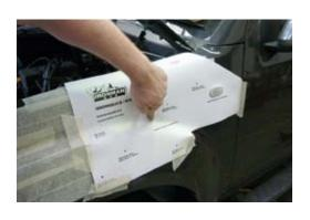
4. Using a felt tipped pen, mark all holes through template onto mudguard. Remove template.
