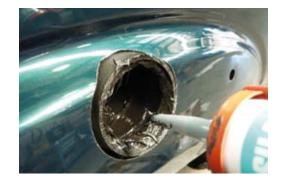
30. Attach snorkel body to mudguard using M8
