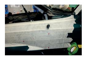
6. Using a 108mm holesaw cut hole for snorkel duct and drill stud mounting holes to 16mm.
