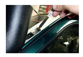
10. Apply silicone sealant to holes and insert mounting plugs.
