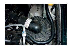
3. Remove air entry duct from between inner and outer mudguards by removing 5 x 6mm bolts and levering away from inner guard to break away adhesive.
