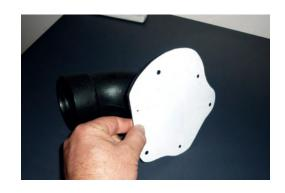
14. Place remaining template on air cleaner flange and mark sections to be removed to allow it to seal against connecting elbow.
