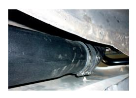
18. Fit elbow from engine bay through inner guard and connect to air entry duct with connection hose. Secure elbow flange to inner guard with M6 Bolts and tighten hose clamps.
