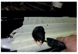
7. Drill all mounting holes to 16mm.
