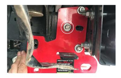
6. Place the spacer plate on the other side of the factory tie down point and use the supplied 10.9 tensile bolt, 2 x flat washers, spring washer and nut.
