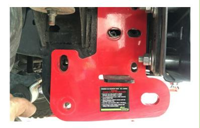
**4.** Re-use the U-bolt from the strengthening bracket and leave loose.
