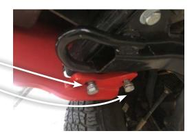
8. Re-use the x 2 bull bar bolts that were removed from step 3.
