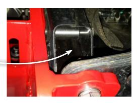
7. Using 2 x M10 bolts, spring washer, and flat washer secure the under side of the recovery point to the tie down point.
