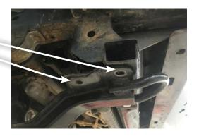
5. Lift Recovery point into position, use the supplied M12 x 100mm bolts, washers and nuts to secure it to through chassis.
