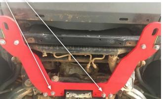
8. Use the 2 x M10 bolts, spring washers, and flat washers in the remaining 2 holes of the recovery point
