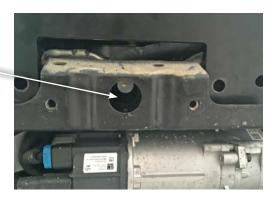
7. Feed the 2 x nut plates with the long wire through the hole, to pick up each of the centre holes of the recovery point using M12 bolts, spring washers and flat washers
