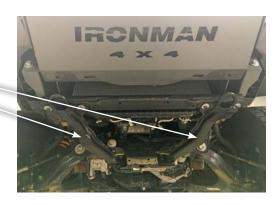
4. Lift recovery point into position. Using 4 x M10 bolts, spring washers, and flat washers, loosly attach recovery points using the holes illustrated.
