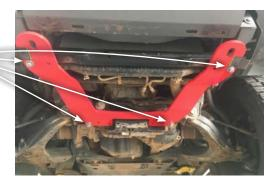
5. Feed the 2 x nut plates with the short wire into the radiator support mount to pick up the front inner holes use 2 x M12 bolts, spring washers and flat washers
