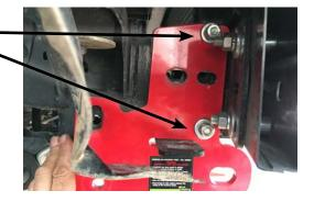
5. Re-use the long bolt, washers and nut removed from bracket, then pass back through the chassis.
