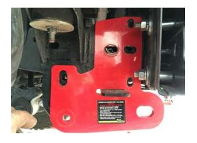
4. Re-use the U-bolt from the strengthening bracket and leave loose.
