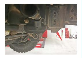
3. Position the Recovery Point to the chassis and use 2 x M10 bolts, flat washers and spring washers. Leave loose.
