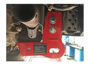
4. Use the M12 long bolt, pass through the chassis vertically through along with the flat washer, spring washer and nut, leave loose.
