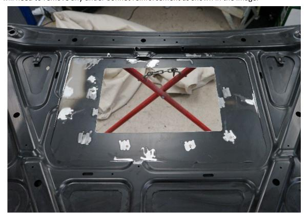
NOTE: This bonnet scoop will need to be sanded to the individual profile of the bonnet as every vehicle can be slightly different. This will ensure a professional finish and give the best durability. Failure to do so will leave a gap between the bonnet and the scoop.
