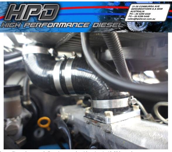
8. Fit 50mm silicone hoses and alloy pipe to turbo side using 4x 40-60 hose clamps.
