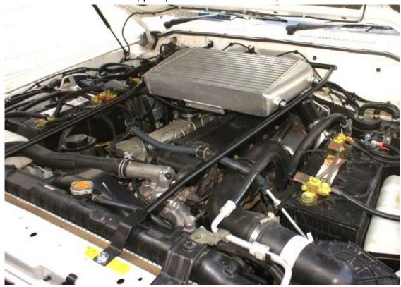
**11.** Fit the 4mm boost hose removed from standard cross over pipe to hose tail on inlet manifold adaptor. This hose is connected to the boost compensator on the top of the injector pump.
