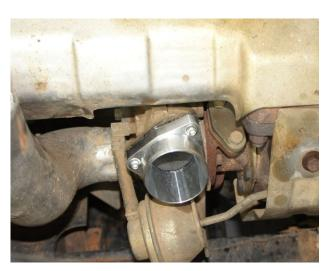
**4.** Bolt rear sub frame to studs on fire wall using 2 x 8mm nuts and washers.
