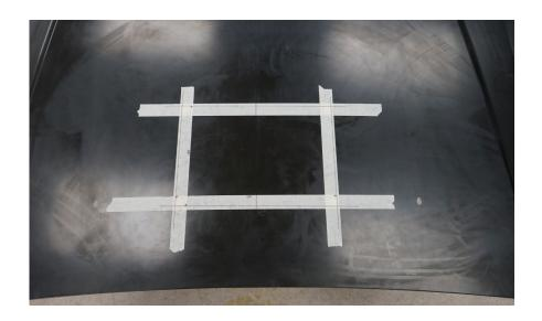
13. Take a measurement from the intercooler core back to the bonnet recess on all 3 sides (driver's side inner guard, passenger side inner guard and below the windscreen) of the intercooler. These marks are your outer core measurements. Your cutting line is 10mm inside the edge of the core. Your overall hole size will be 415 wide x 280mm deep.
