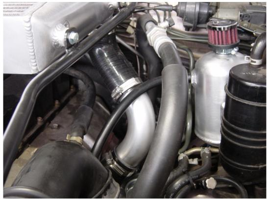
9. Bolt the front driver's side intercooler frame to radiator support panel with m8x25 bolt and washer
