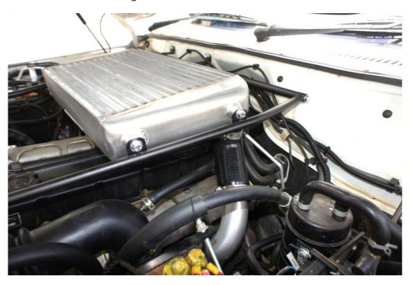
7. Fit 2x 63mm 90deg silicone hoses between inlet manifold and intercooler using alloy joiner pipe and 4x 60-80 clamps, you may have to trim the silicone hoses to get the correct fit.
