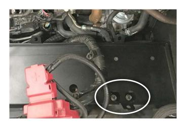
8. Place the 2 x M8 bolts, spring washer, and flat washers in the next 2 x holes. Plus the countersunk M8 bolt in the front most hole, and leave loose.
