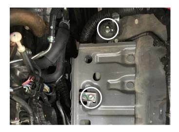
4. Remove the 3 x bolts and 3 x nuts from the inside of the guard as shown, and disregard.
