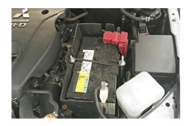
3. Undo the 2 x M6 bolts that hold the factory loom, and remove the steel brackets.
