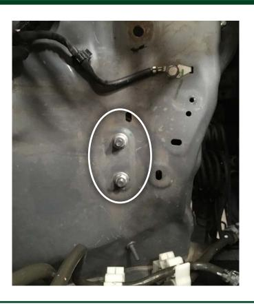
6. Loosely attach the rear plate using the 2 x M6 countersunk bolts and feed tray underneath the factory loom.
