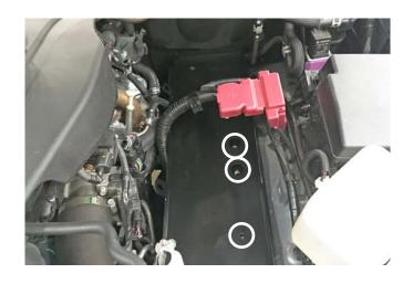
9. Feed the 3 x bolts, spring washers and flat washers through the inner guard towards the engine bay, and use 3 x nuts and leave loose.
