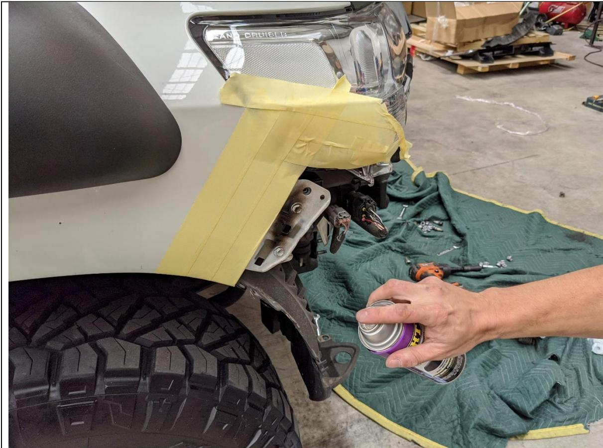
33. On vehicles with light colour paint, such as the car shown. It is recommended to paint the under headlight areas that will be visible through bar clearance gaps and mesh panels.
