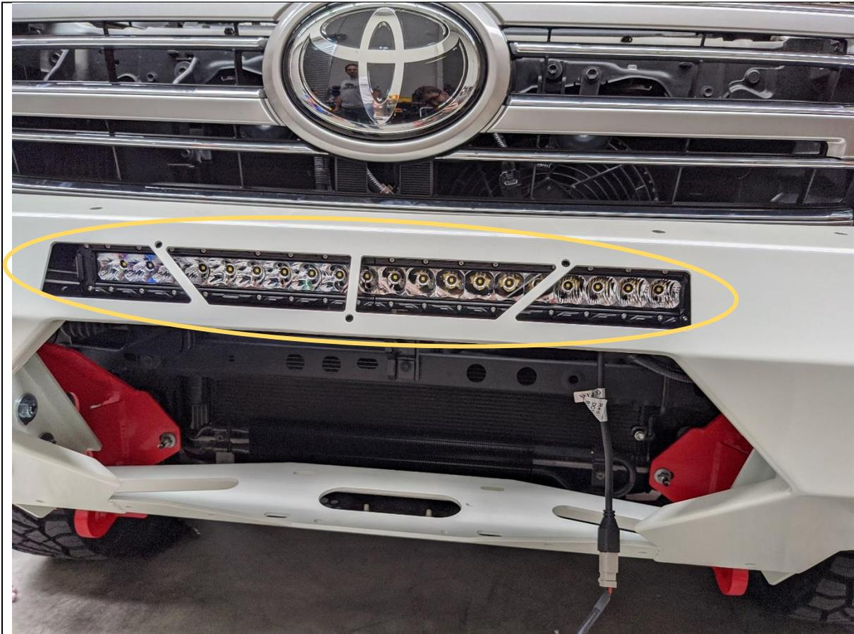
66. If Fitting an integrated light bar, do so now. Leave bolts loose at this stage to allow fitment of mesh panels.
