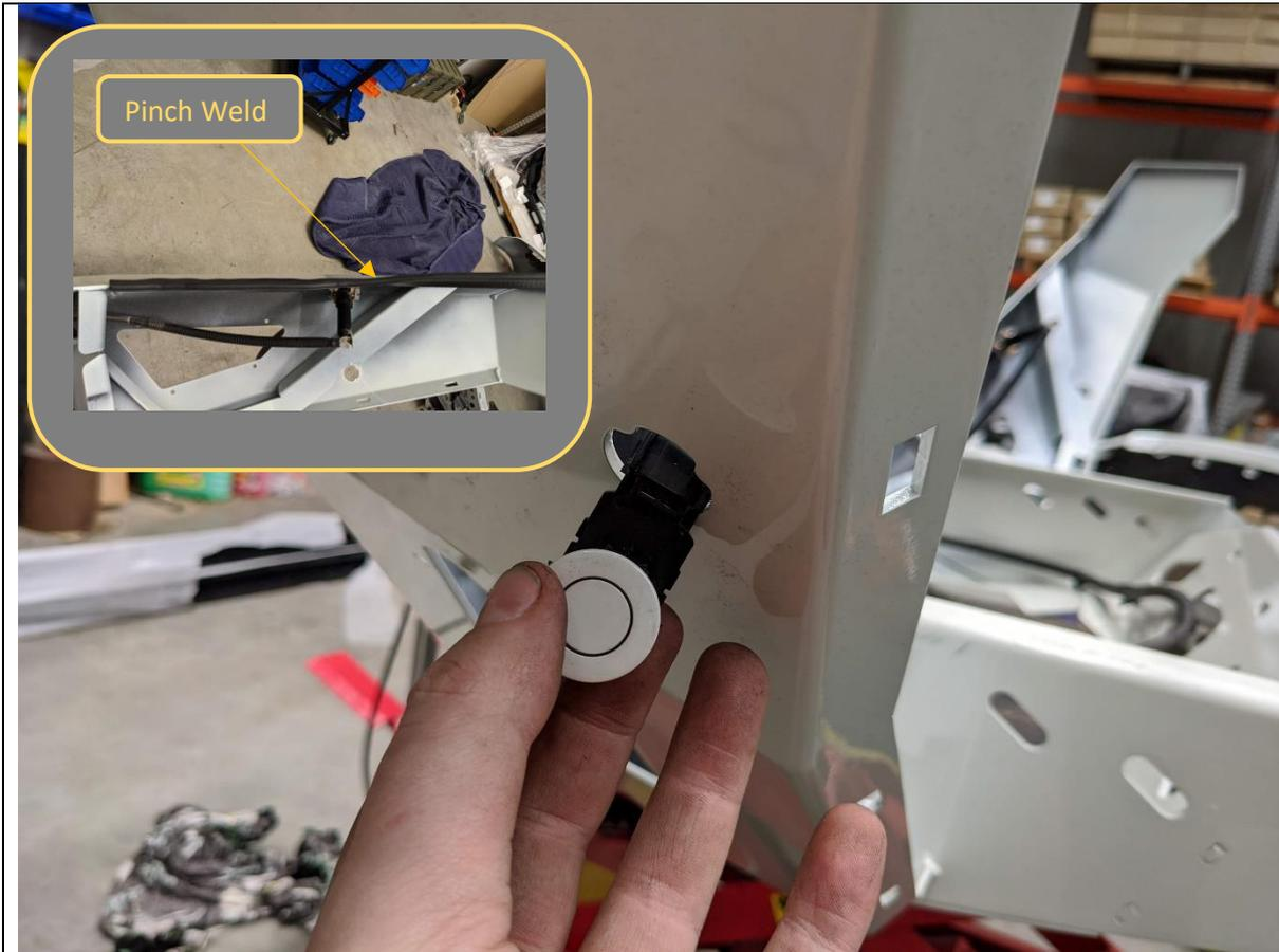
59. Re Fit parking sensors to the bar. Insert the sensor from the front of the bar. Push the sensor through and allow the tabs to expand and hold the sensor in place.
