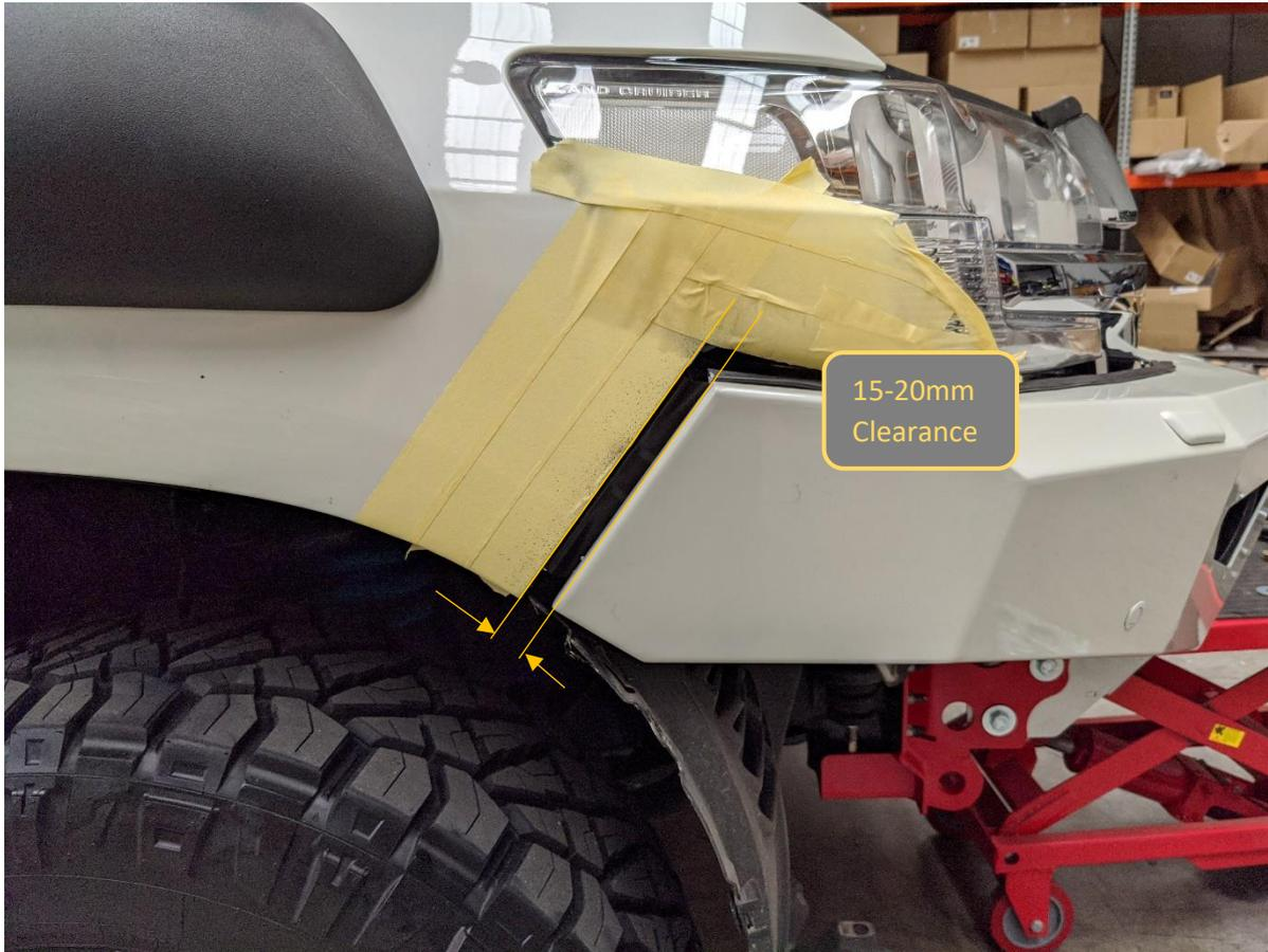
64. With assistance, either from another person, Align the bar with the edges of the vehicle. Adjust such that the clearances are neat and even side to side.
