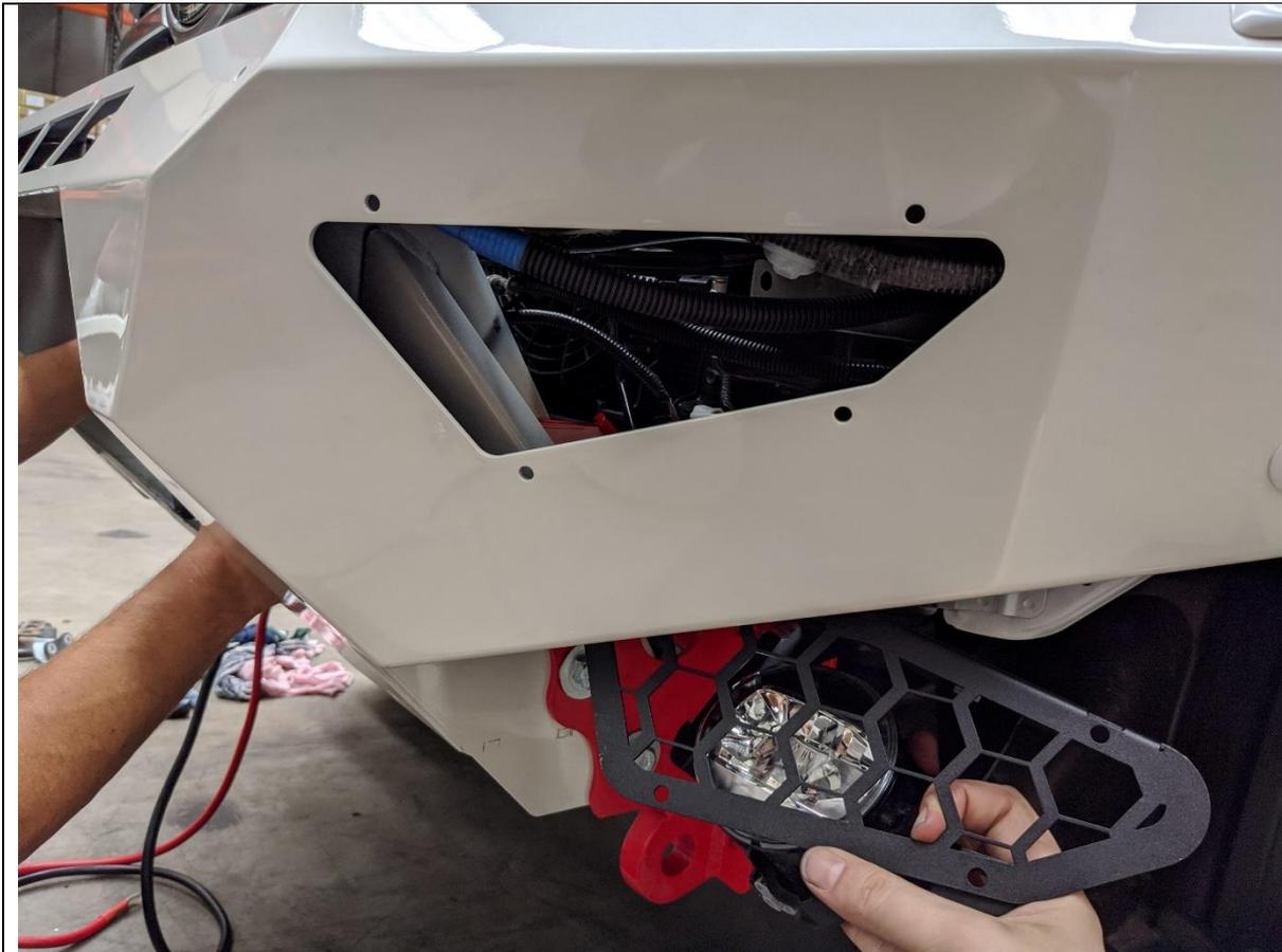
82. Fit Light cover mesh to bar using 4x M6x16 Button head bolts, Flat washers and M6 Flange Nuts
