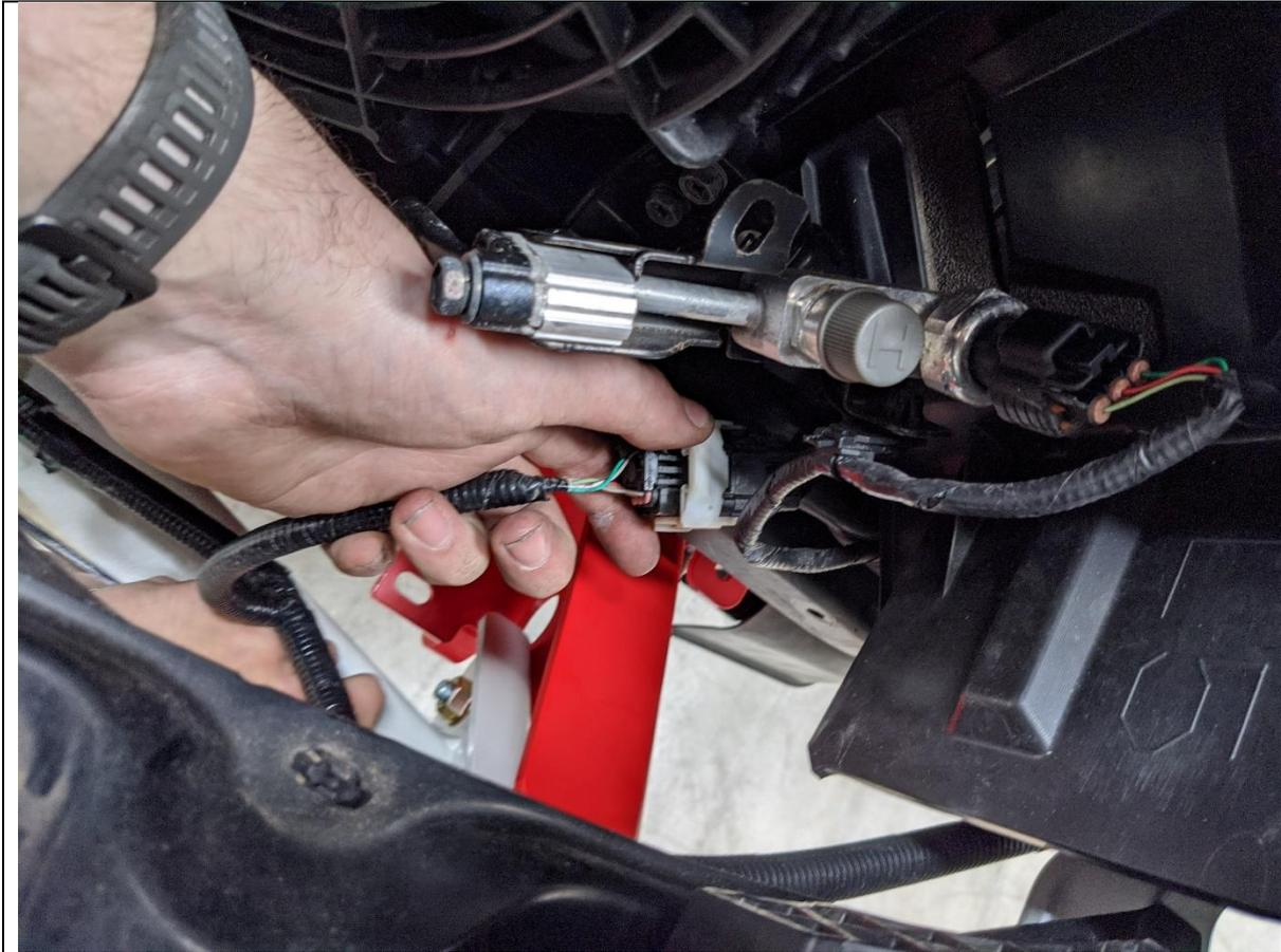
84. Re Connect Electrical Harness and headlight washers behind grille. If equipped also reconnect Radar and Camera harnesses.
