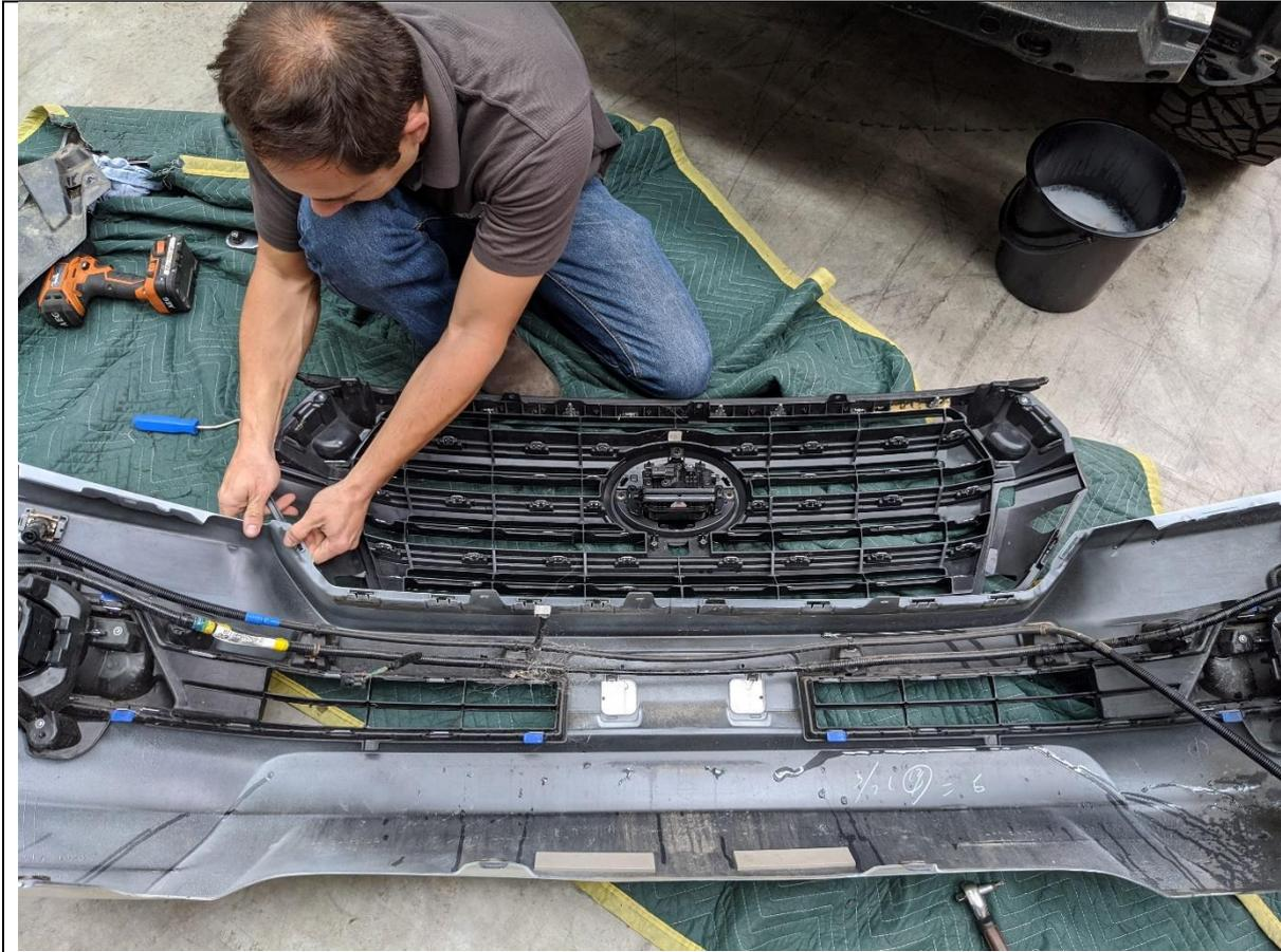
16. Remove the grille from the bumper by pinching and pushing forward the clips securing the bottom edge of grille to bumper.
