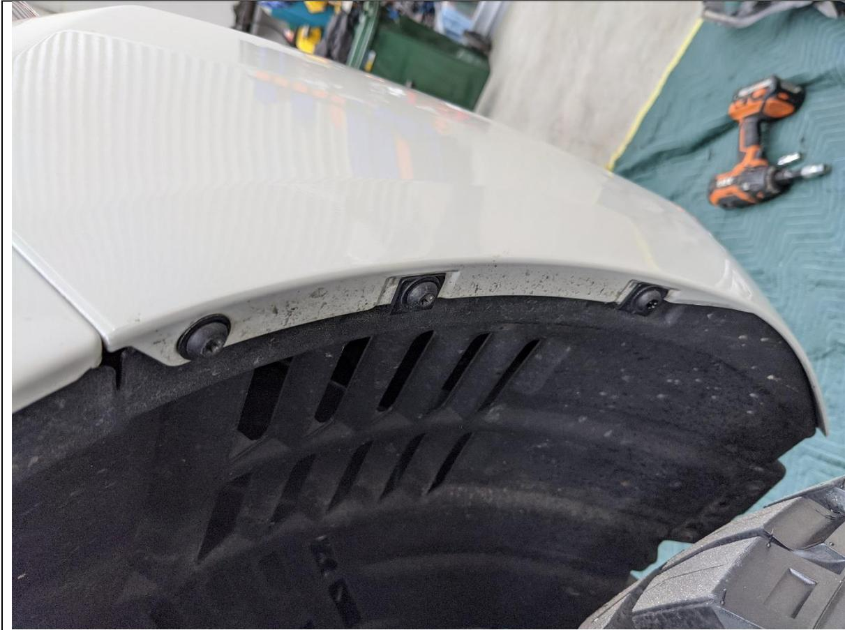
9. Remove the T30 Torx screws securing bumper to the wheel arch liner.
