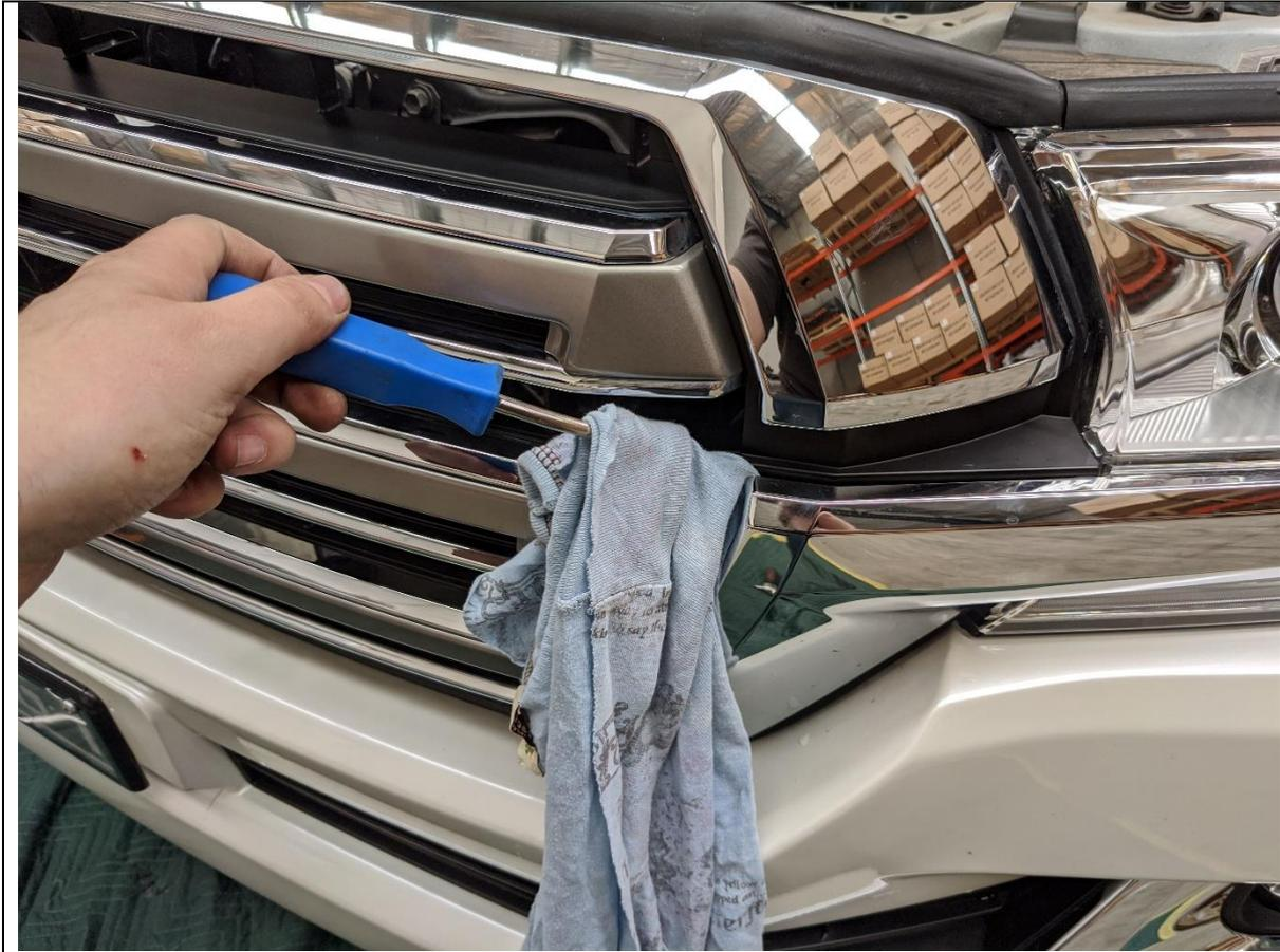
5. Using a rag to protect the chrome finish, carefully pry the L shape headlight trim to release the clips.
