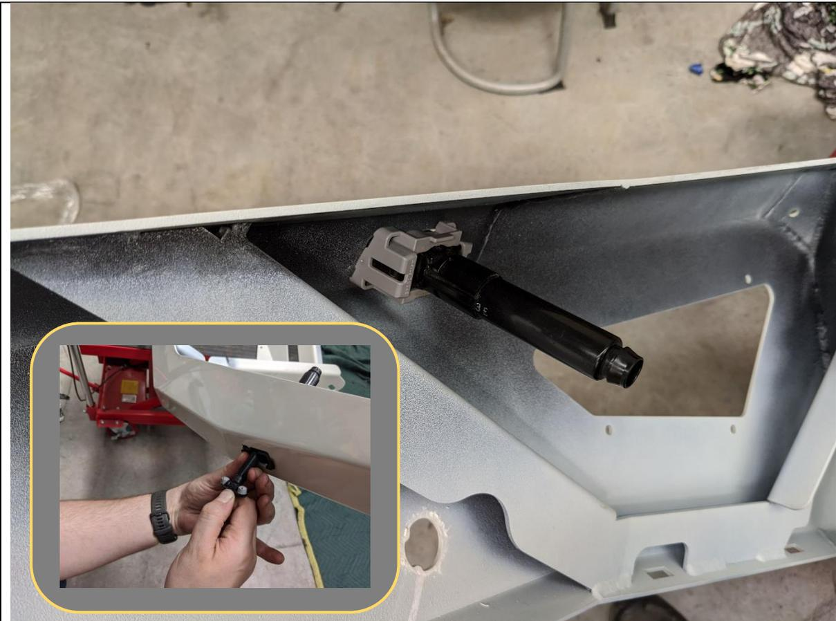
56. If Equipped Re fit headlight washers to bar.
