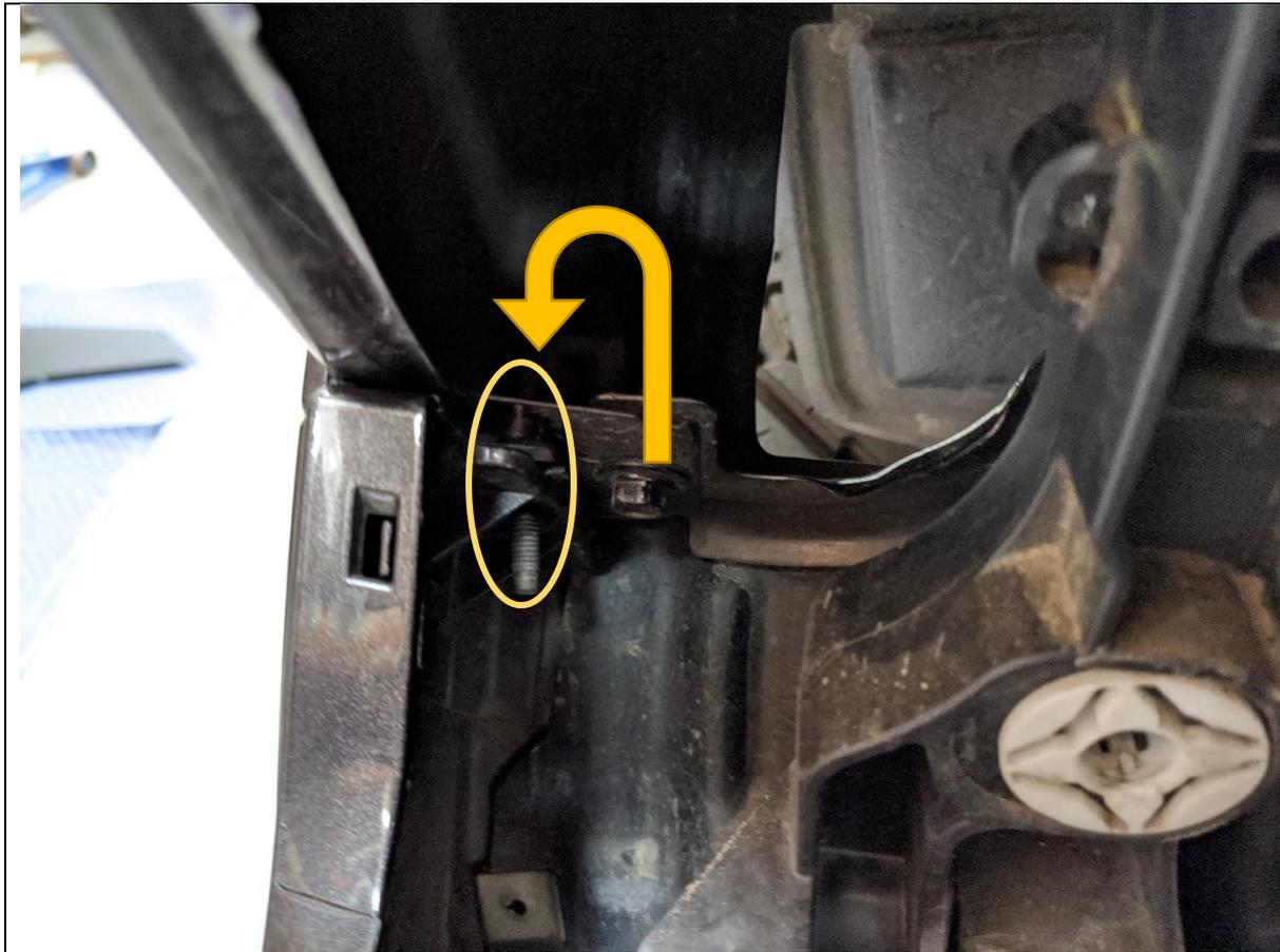
14. With access through the headlight opening, remove the 10mm head bolt securing the upper bumper trim.
