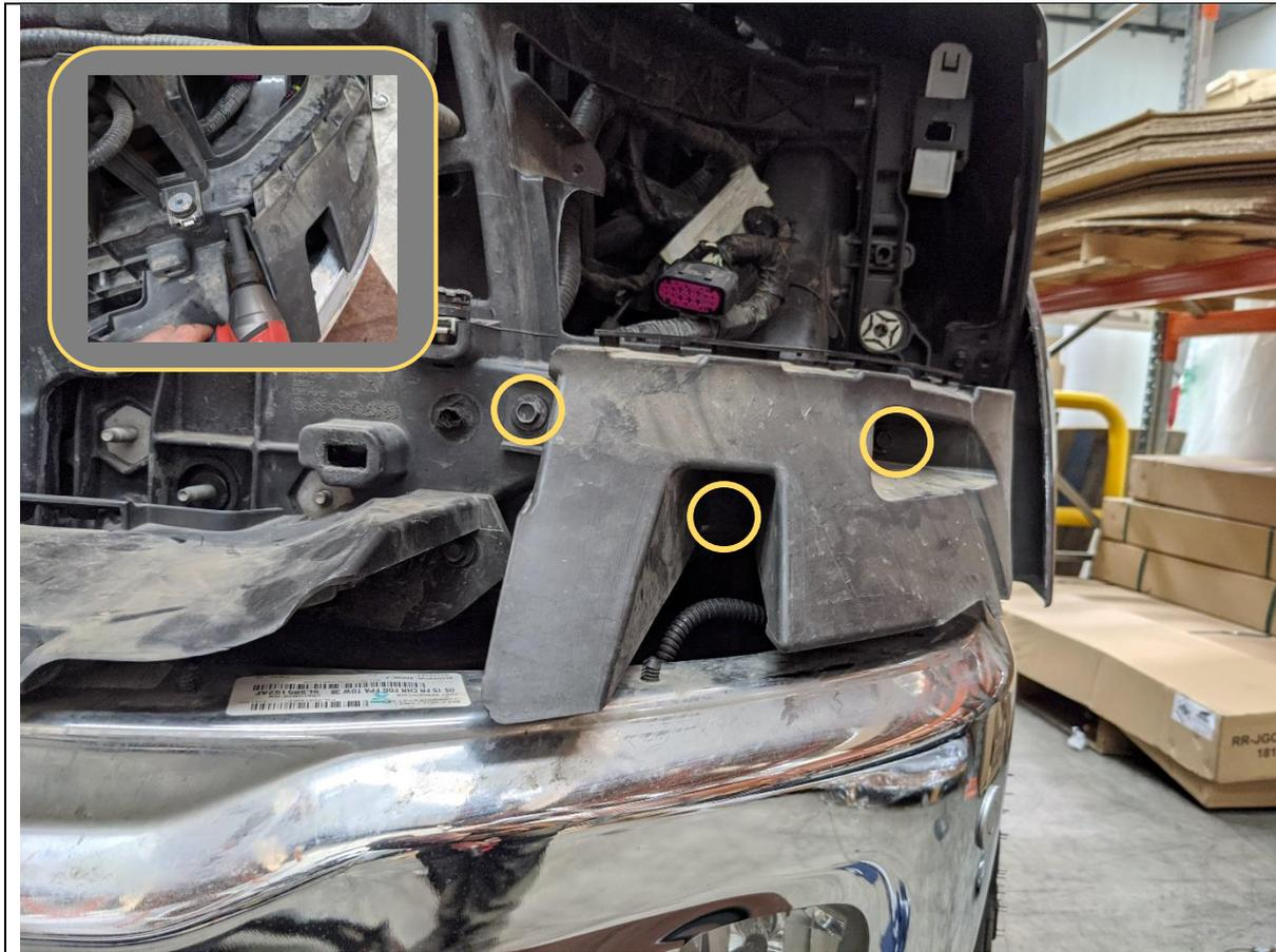
20. Remove the outer plastic bumper supports by removing the 3x 10mm head screws securing it to the crossmember.
