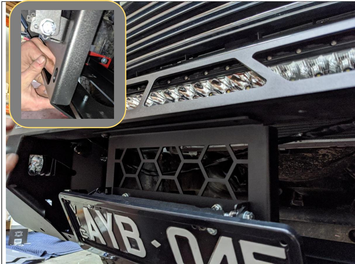
87. Fit the Mesh Fairlead Mount to the center of the bar, using M8x16 Button head (Top), M8x20 Button Head (Bottom) M8 Flat washers and M8 Flange Nuts.
