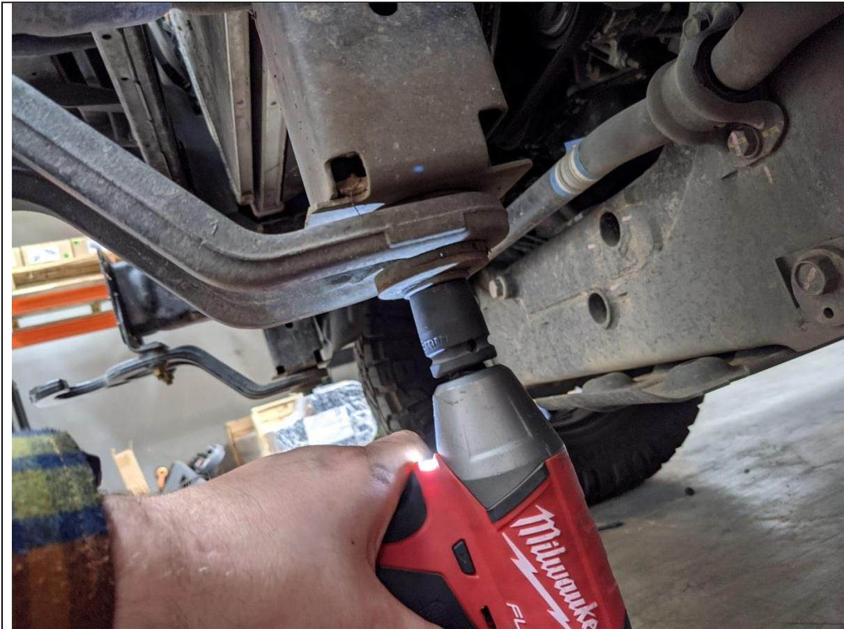
30. Remove the factory tow hooks, by removing the M12 Fine pitch bolt securing it to the chassis.
