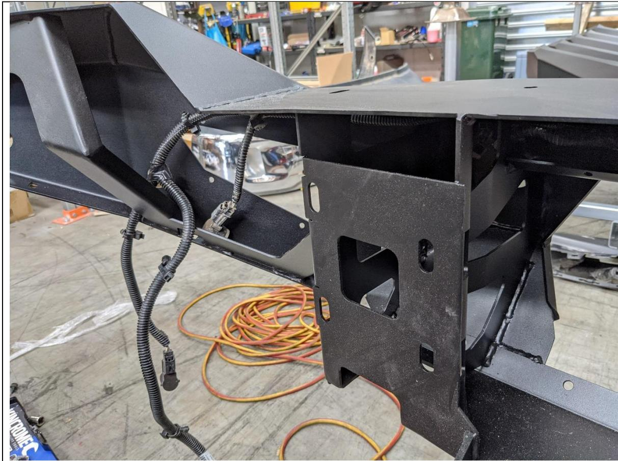
50. Pass wiring loom through bar uprights, starting from the left-hand side of the bar.
