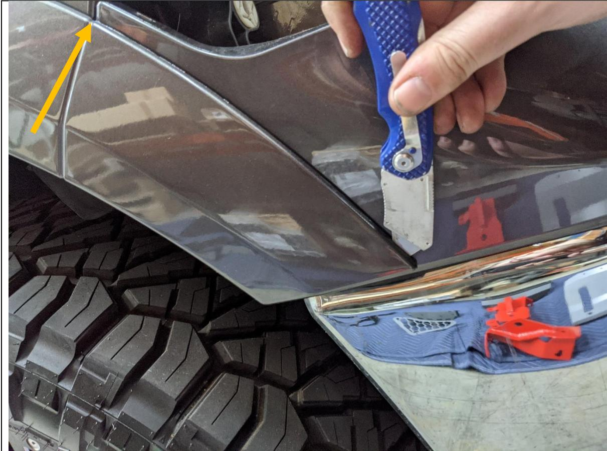
16. Using a Utility knife carefully cut the double-sided adhesive tape securing the wheel arch flare back to the bumper to guard joint in the body.
