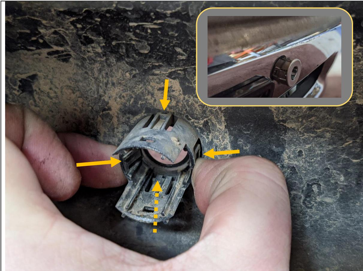
35. Remove sensor housings from front bumper. Squeeze on the 4x retaining tabs whilst pushing housing from back side of bar to release.
