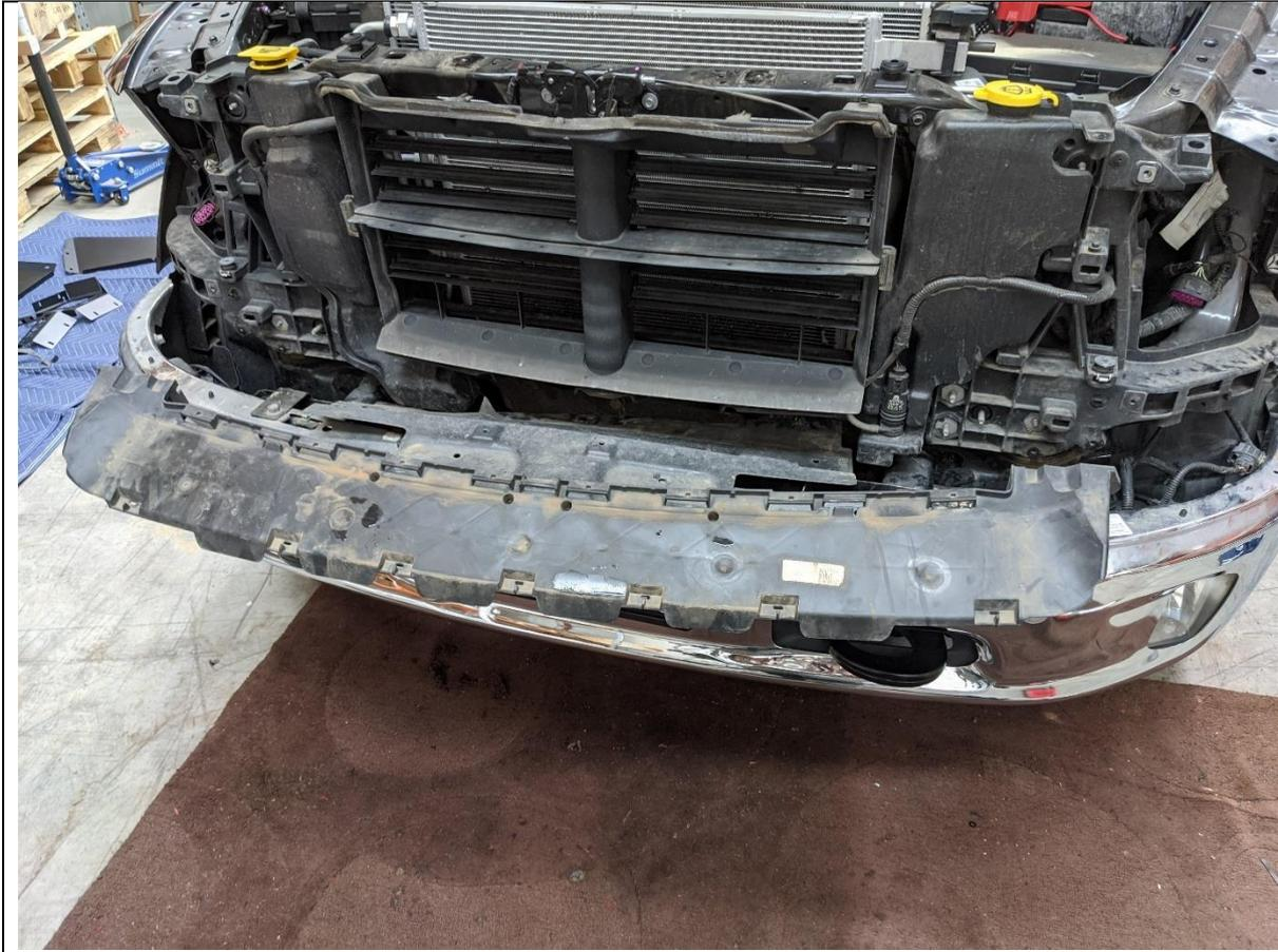
24. Remove the upper bumper support and air guide.
