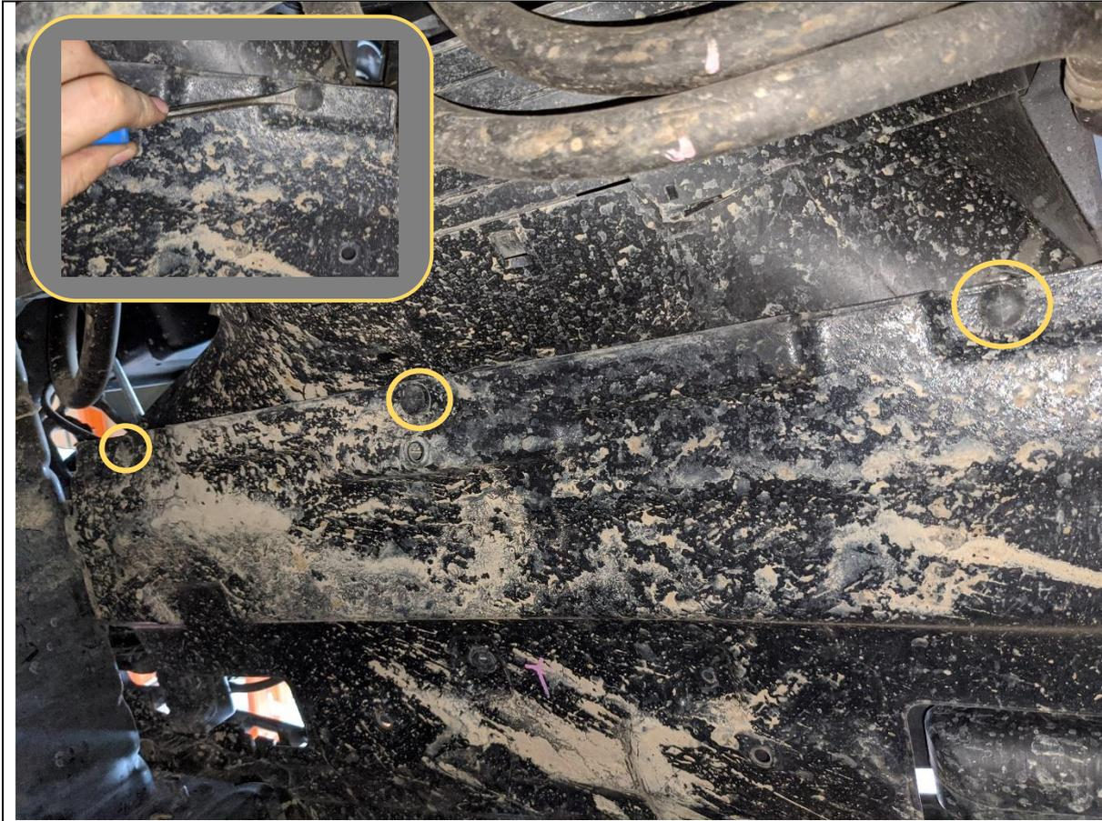
23. From underneath the car, remove the 3x Xmas Tree clips that secure the air guide from the radiator shroud using a trim tool.
