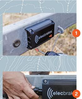
Fasten the unit to the draw bar using the mounting screws provided.
