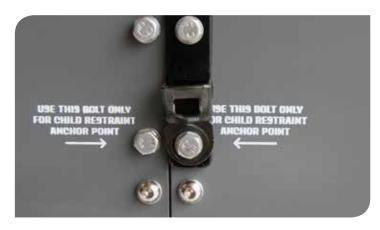
The same second bolt down from the top only can be used as a Cargo Barrier mount and a Child Restraint point from the same bolt if needed. (see image above)
