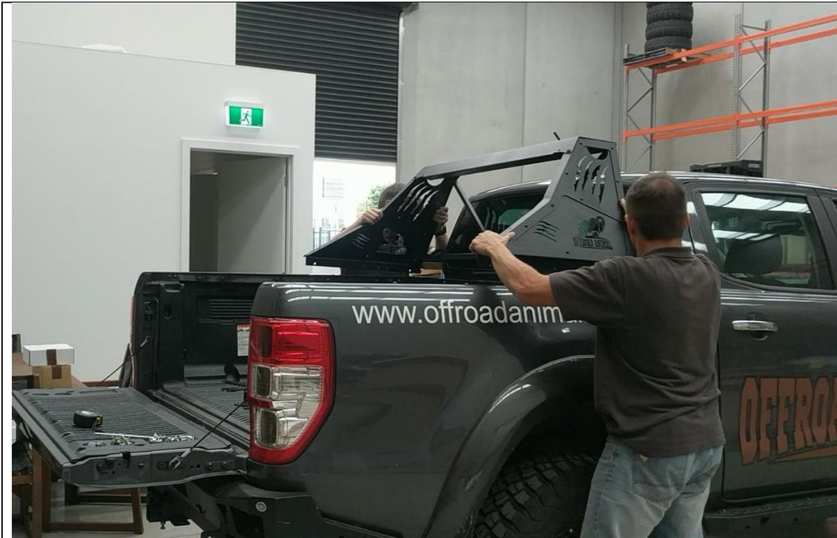
6. With assistance, Lift the assembled chase rack onto the bed of the ute.
