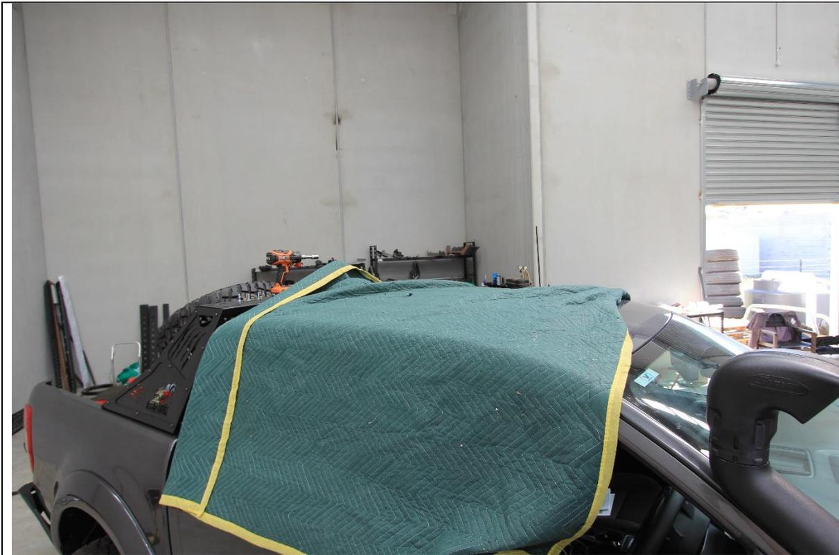
8. Prepare vehicle roof, by covering with a blanket or other soft protection sheet to prevent marking of roof.
