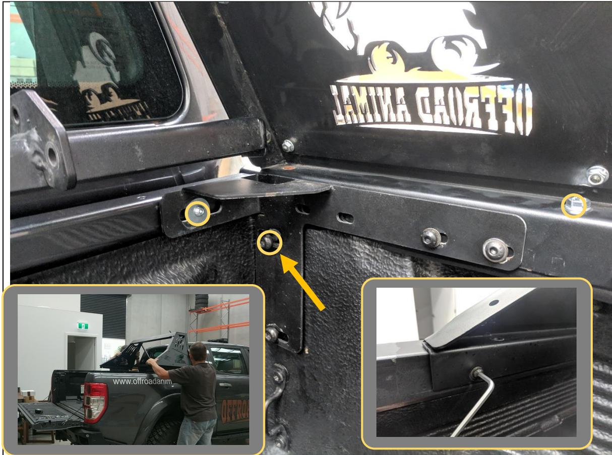
13. With assistance Re-fit chase rack to tub and align with holes drilled.
