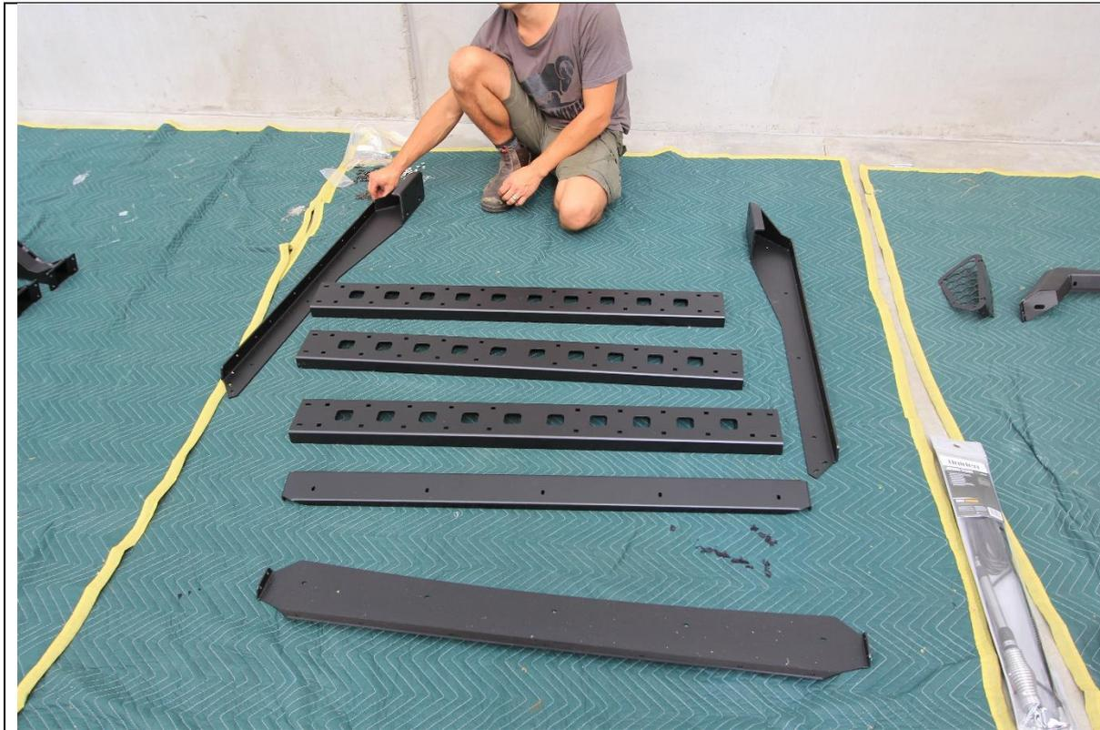
3. Start by assembling the roof rack on the ground, away from the vehicle.
