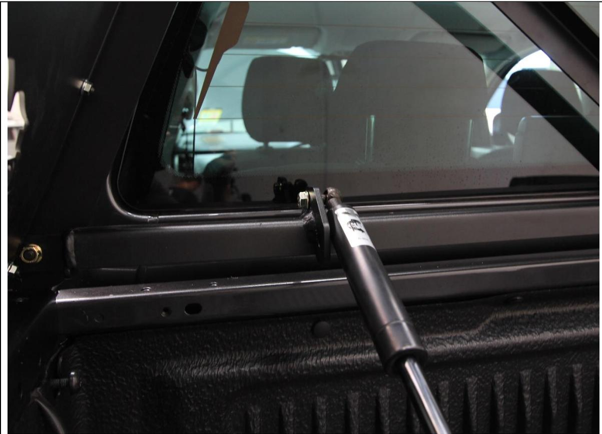
5. Fit the gas struts to the tie bar, using M8 Flange nuts.
