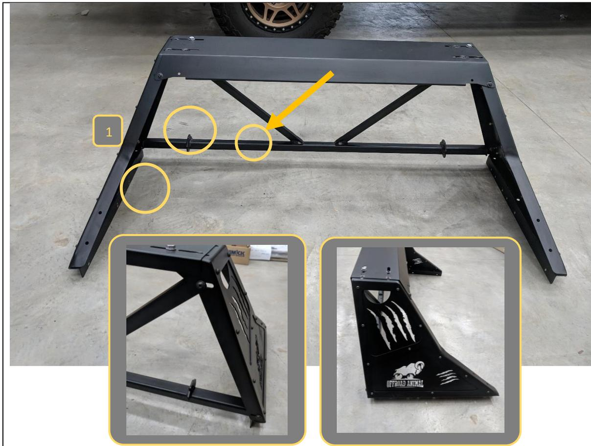
1. Start by assembling the Chase rack on the ground, away from the vehicle.
