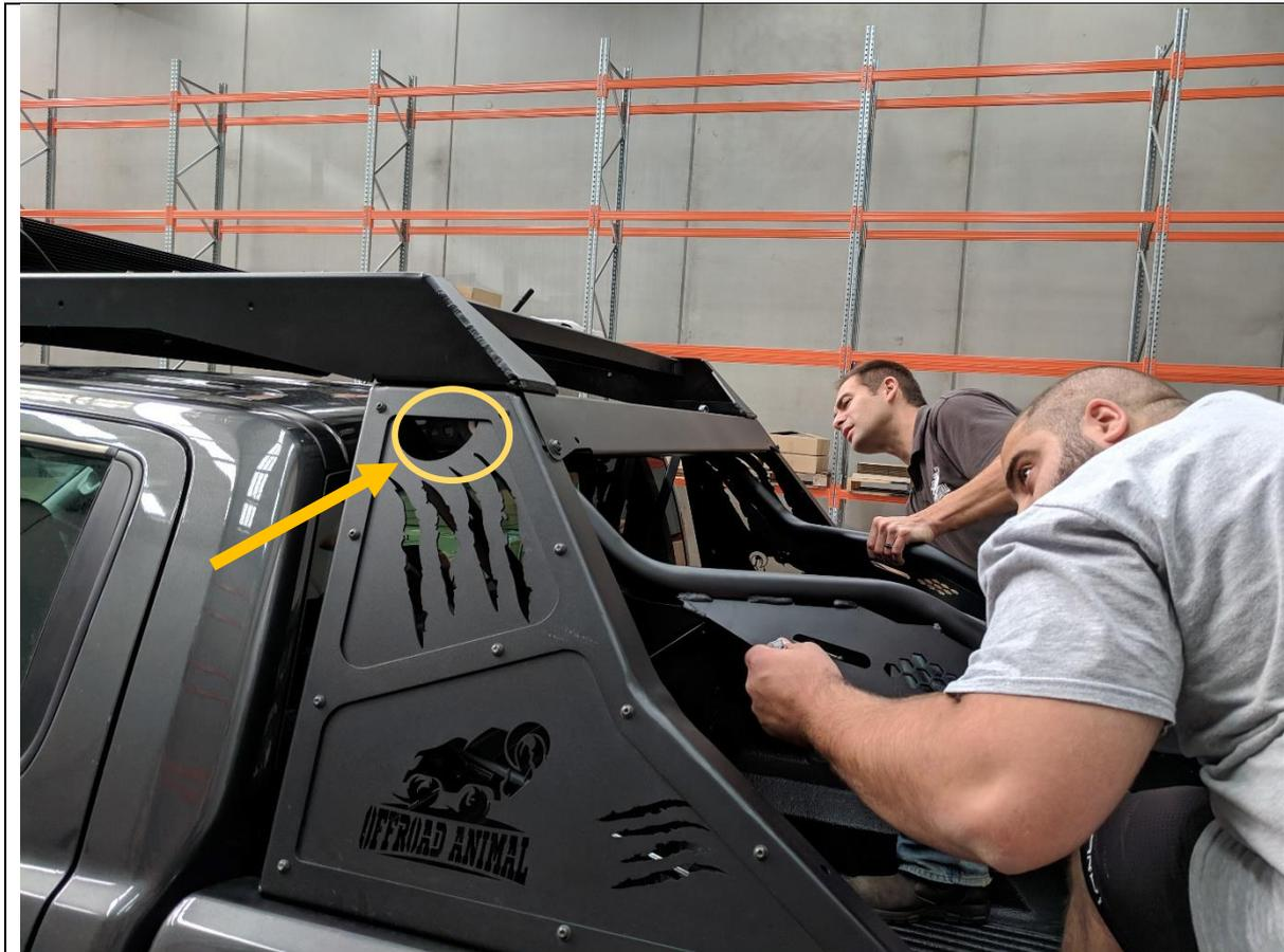
11. With assistance lift the tire carrier assembly and align with the support brackets.
