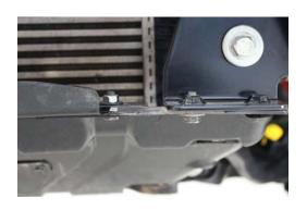
17. Fit protection plates using M8 bolts and hardware provided.
