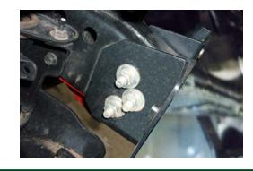
7. Fit winch cradle to front of vehicle. Do not tighten the bolts at this stage as adjustment will be required once bar is installed.
