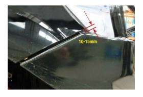
13. Drill and pin bar into position using M10 bolts, washers and nuts supplied.
