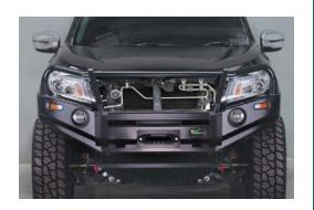
12. Align bull bar with vehicle ensuring there is a 10mm to 15mm gap between wing of bull bar and mudguard. Tighten all bolts.
