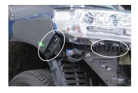
3. Cut plastic air-deflectors along lines as shown to allow fitment of bull bar to bracket
