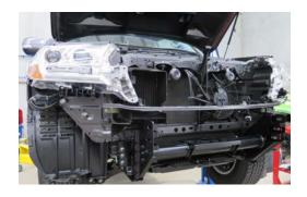
5. Insert threaded anchor plate supplied, into the rectangle shaped hole in the side of the chassis as shown in pic A.
