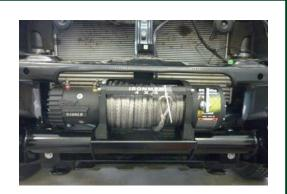
19. Fit bull bar to chassis brackets using M12 bolts, flat washers, spring washers and nuts provided.
