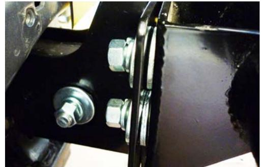
6. Using holes in inner and outer of chassis strengthening brackets as a guide, drill a 12.5mm hole and install a mounting bolt washer, spring washer and nut. Tighten all bolts.
