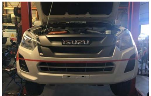
8. Using an air hack saw or similar, cut along line previously marked to remove the lower section of the bumper bar.
