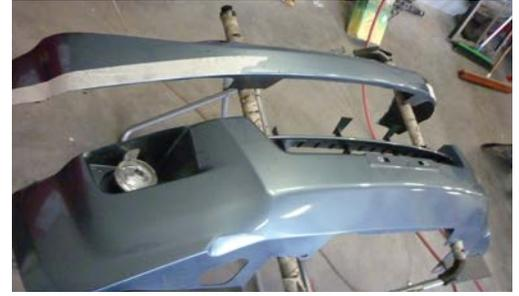
9. Place cutting template on the ends of the bumper and mark as shown.
