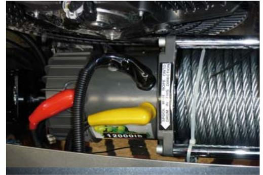
25. Connect the thin black earth wire and negative battery cable to the earth connection on the opposite side of winch motor.
