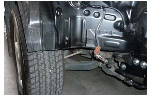
5. Install winch cradle and chassis strengthening brackets as shown using hardware provided.
