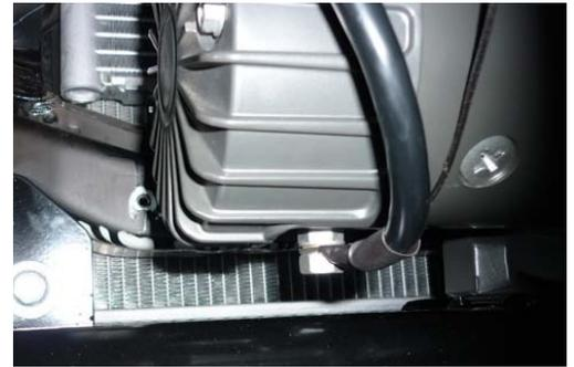
26. Run the positive and negative battery cables into the engine bay taking care to secure cables away from any sharp or moving objects.
