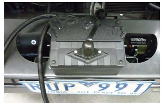
24. Connect three colour coded cables to the corresponding poles on winch motor.
