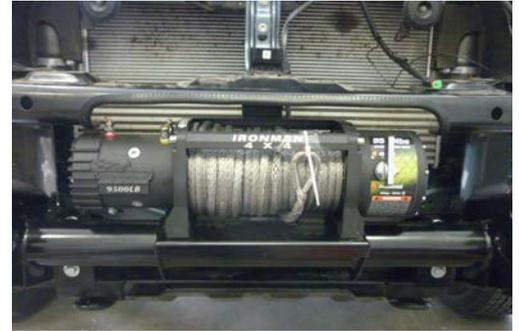
14. Refit top section of bumper bar to vehicle using original clips.
