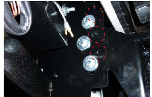
22. Bolt fairlead to recess in front of bull bar using bolts, washers and nuts provided.
