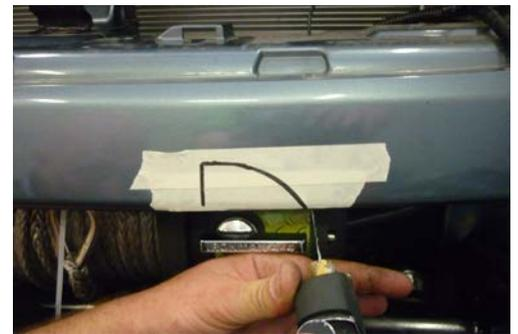
16. Cut return from bumper bar to allow clearance for the winch as shown.
