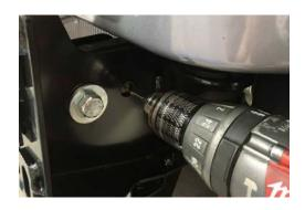
7. Install winch cradle as shown using hardware provided.
