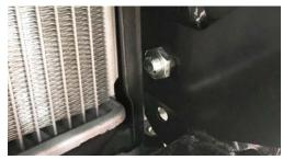
6. Using holes in inner and outer of chassis strengthening brackets as a guide, drill a 12.5mm hole and install a mounting bolt washer, spring washer and nut. Tighten all bolts.
