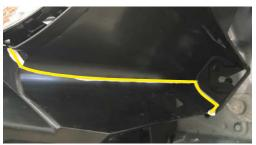
NOTE: Make sure that attaching hole remains on grill as shown.
