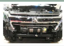
10. Remove protuding sections from below headlights as shown.
