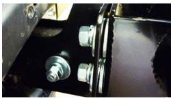
NOTE: Check bolt clearance on radiator.
