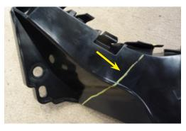
8. Mask lower edge of guard and paint lower section satin black as shown.
