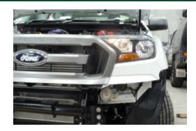
7. Remove bumper and plastic bumper support brackets. Cut along marked line as shown.
