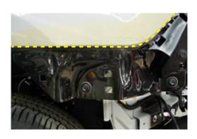
9. Re-fit plastic bumper bar support brackets as shown.
