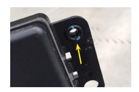
6. Temporarily re-fit top section of bumper bar (cut in previous step) to vehicle. Using end of bumper bar as a guide, mark cut lines onto plastic bumper support brackets.
