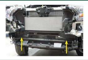
11. Mark up cut lines on passenger side of air duct shields following the edges and contours of the shield as shown in pic A.
