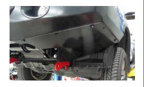
18. Trim guard liners using protection plates as a guide.
