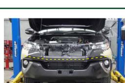
5. Remove grill, front bumper bar, bumper reinforcement and lower bumper support brackets.
