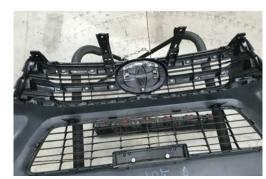
Refit grill using supplied bracket to secure centre section as shown.
