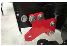
4. Install chassis bracket to vehicle using hardware provided as shown.
