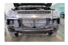
4. Remove bumper bar reinforcement.
