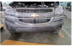
3. Cut along line marked in previous step to remove lower section of bumper bar.
