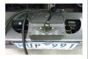
24. Connect three colour coded cables to the corresponding poles on winch motor.
